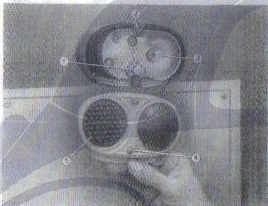
Fig. 66. - Opening the tail and braking lamp.
